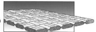
Mat with slab construction, and two-dimensional pliability for very soft subgrades.
