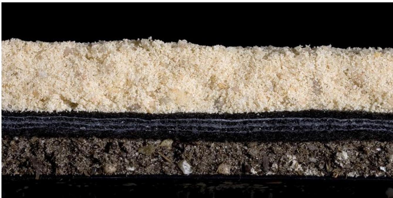
Cross section of a typical FilterMat™ installation with a sand layer placed above the FilterMat™
