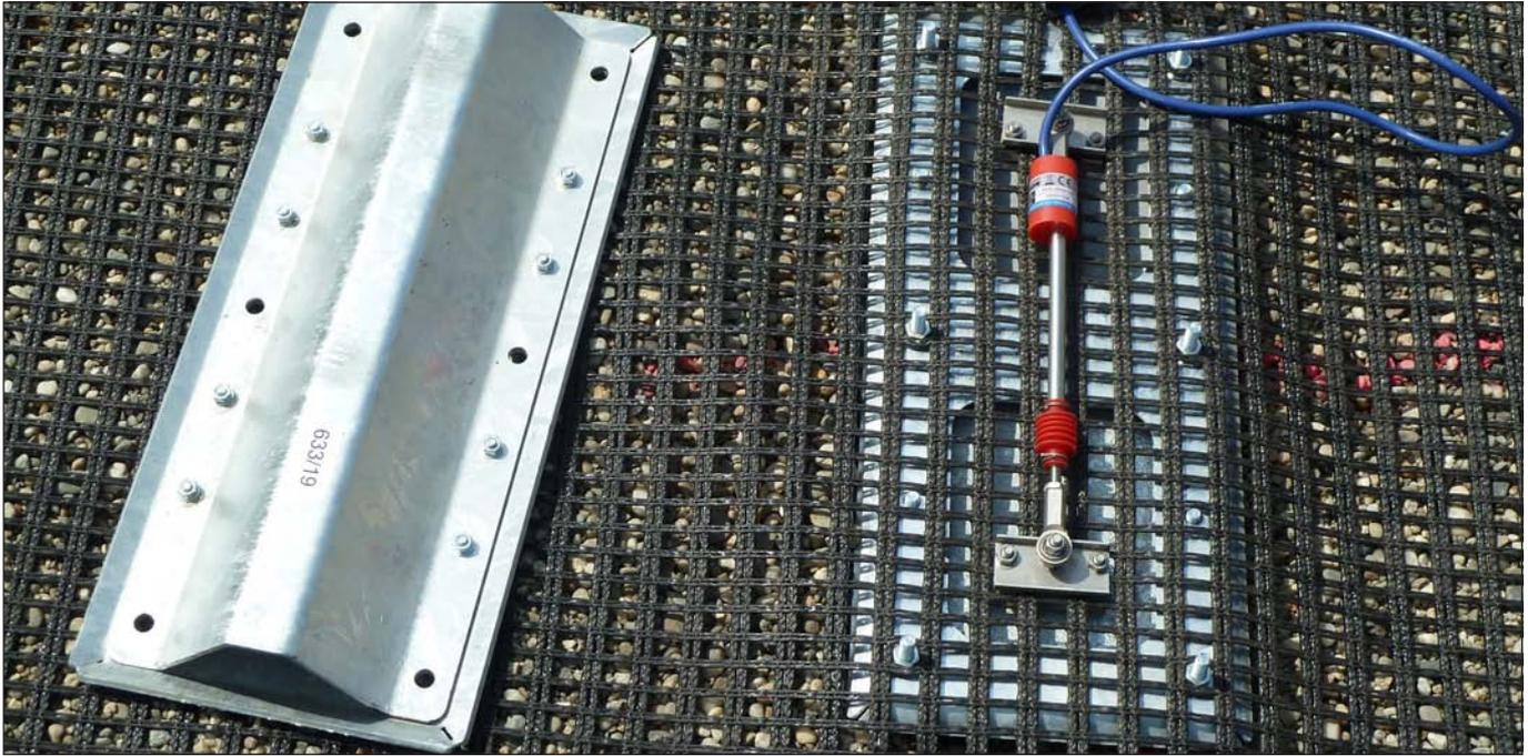
Fig. 12: 2<sup>nd</sup> Monitoring system on Fortrac® geogrid, system NeoStrain®
