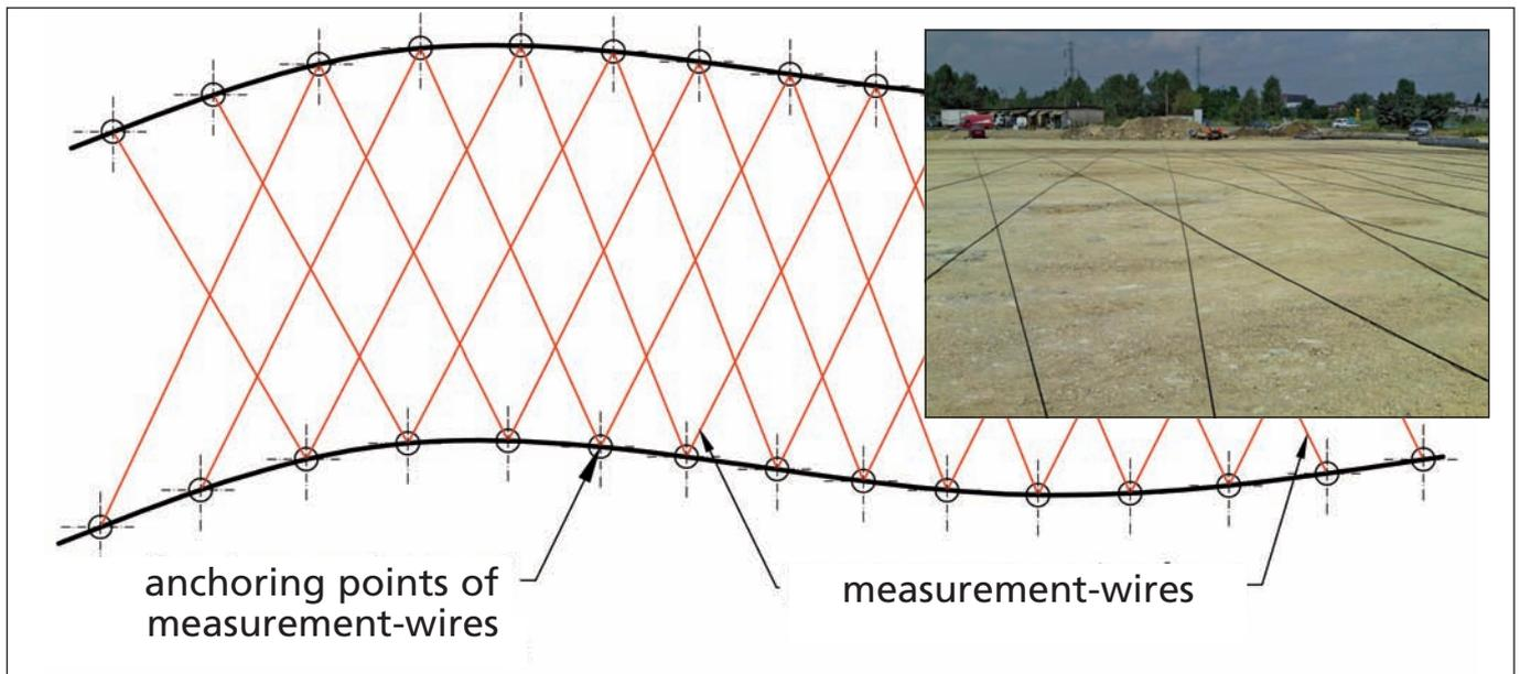
Fig. 10: 1<sup>st</sup> monitoring system (warning layers) diagonal installed measurement wires, System NeoStrain®
