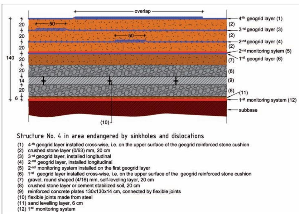
Fig. 9: Designed cross section, structure no. 4
