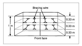
Provide internal horizontal bracing wire at 0.33 m vertical centres in 1 m deep gabions, at the ratio of four wires per cubic metre, see sketch above.
