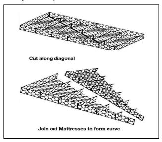
Mattresses can also be cut and folded to form difficult curves. One such technique is shown in the sketch above where the mattress is cut diagonally to form two triangular sections that can be wired together to form a curve.
