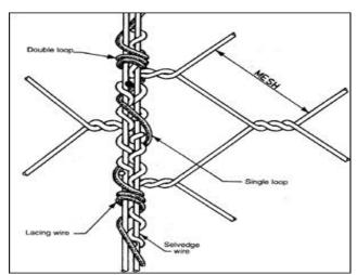
twisting the end of the lacing wire around the selvedges, then lacing around the two edges being joined, using a double tie through each mesh in turn, and tie off securely at the bottom, see sketch above.
