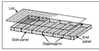
Assemble each mattress individually by raising the sides, ends and diaphragms. The various elements of a mattress are shown in sketch above.
