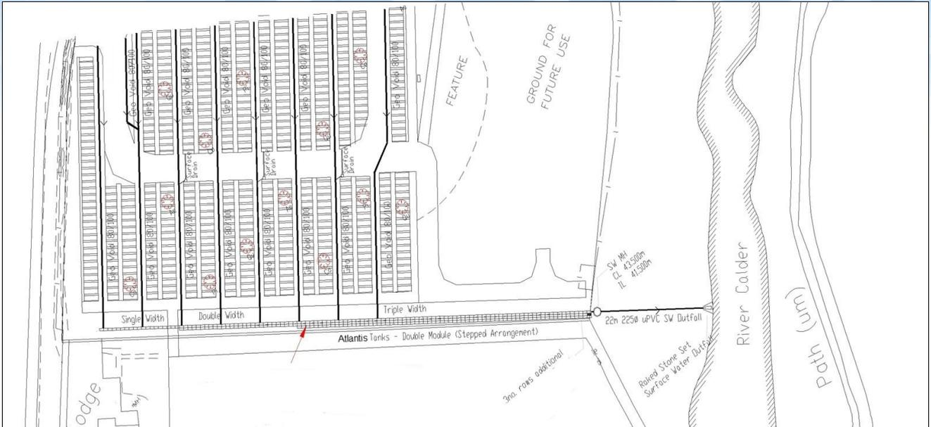
Figure 1. Plan of Lochwinnoch Cemetery including Flo-Pipe and Atlantis Matrix Tank modules
