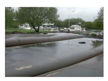
while excess water is released through the pores of the material. In addition, it encourages the formation of a filter cake on the inside of the tube, which in turn limits the discharge of fine particles. **SoilTain®** dewatering tubes are therefore an efficient and effective component for sludge dewatering.
